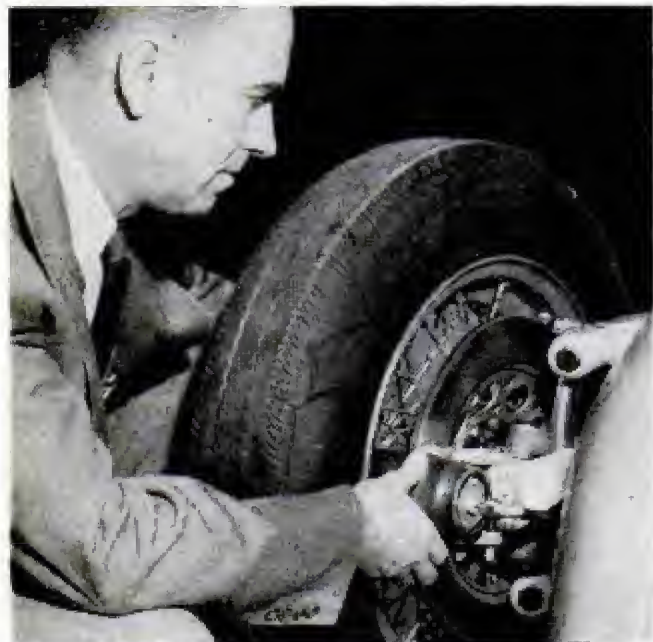
Spot brakes to be used this year consist of two cylinders which clamp the opposite sides of a steel disk
